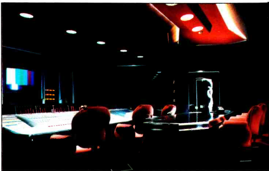
The Editel New York sound mix room, designed by Vin Gizzi, includes the Solid State Logic SSL 6000 with 32 inputs and six mix buses. Expandable to 48 inputs, the Events Controller handles automated dynamic mixing from stored and organized titles, cues and SMPTE locations.
